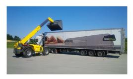
Pre-packed bulk bags - Max  $66m^3$  Walking floor truck -  $18m \times 2.5m \times 4m$
