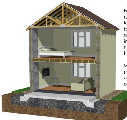
Foundation system using GEOCELL recycled foam glass gravel to form a load bearing, thermally insulated foundation. This simple solution offers substantial advantages including high insulation values and fast construction times which are cost saving, as well as being sustainable.
