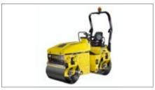
Compaction Factor 1.6:1 Vibrating roller with 2500 kg operating weight
