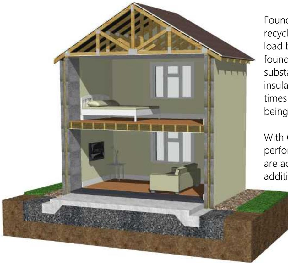
Foundation system using GEOCELL recycled foam glass gravel to form a load bearing, thermally insulated foundation. This simple solution offers substantial advantages including high insulation values and fast construction times which are cost saving, as well as being sustainable.
