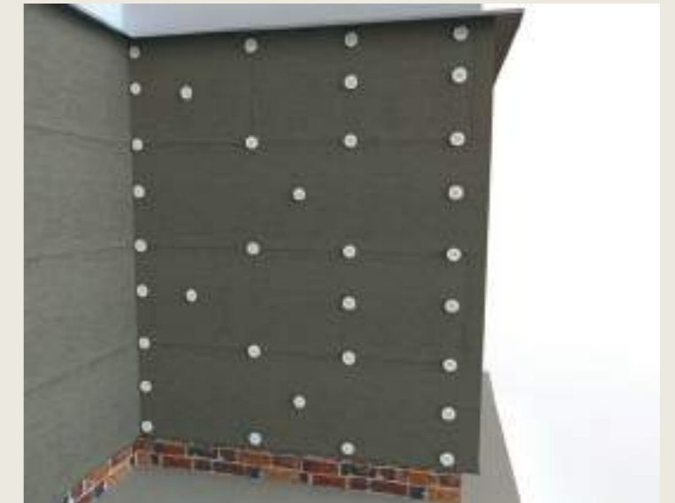
External wall corner
